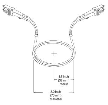
Figure 25. Bending and looping specifications for fiber-optic cables
